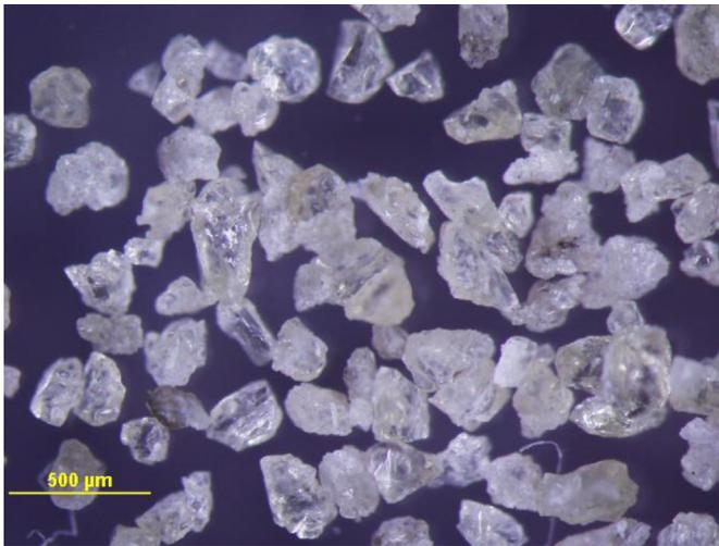
**Fig. 1.** Pyroxenes of the CRONUS-P reference material produced from the NXP 93\*52 sample. Minerals appear clean, without accessory mineral inclusions.
