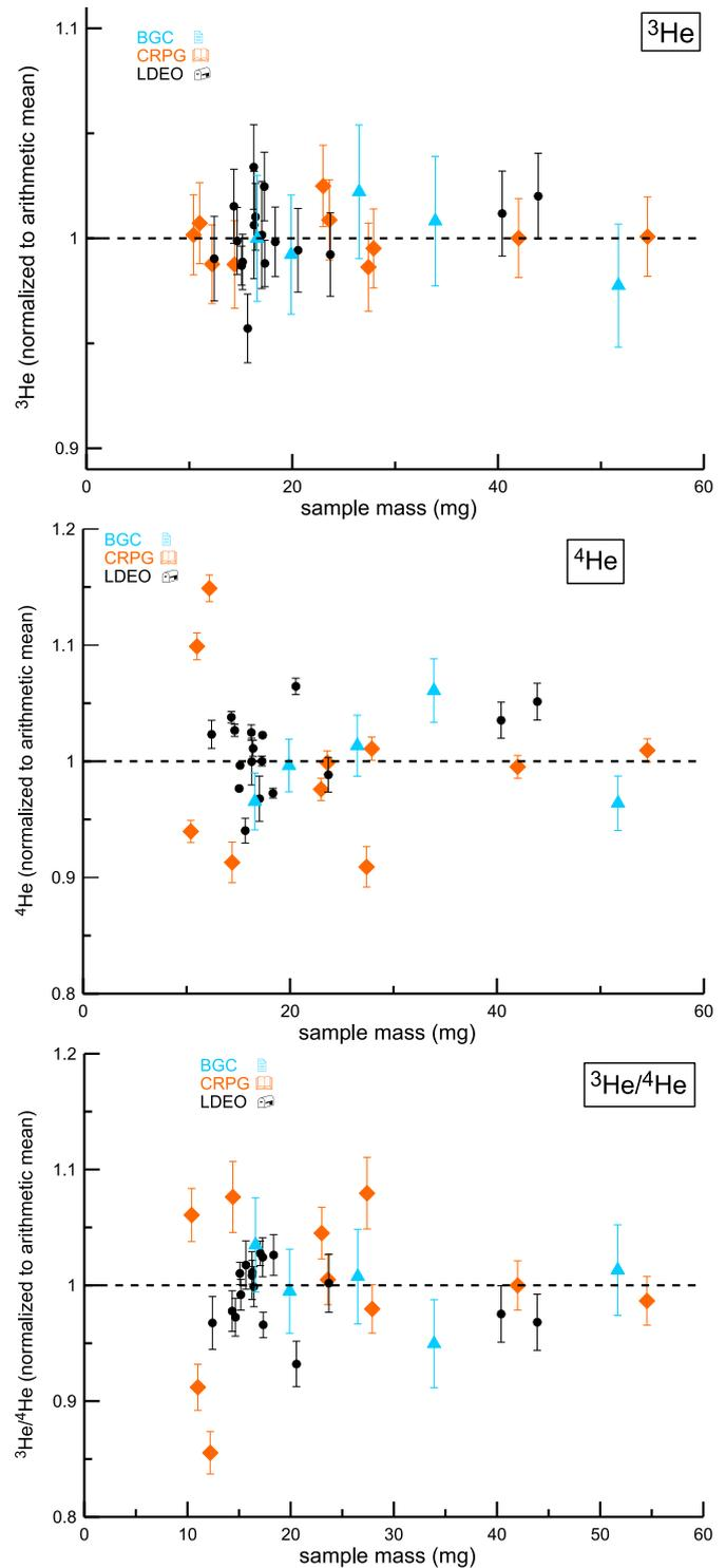
**Fig. 2.** CRONUS-P helium isotope data with  $1\sigma$  errors (normalized per laboratory to the respective arithmetic mean) as a function of sample mass. See Blard et al. 2015 for full data details of an inter-laboratory data comparison.
